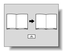
11 If the fold position is shifted to the right, touch to specify the desired negative adjustment (between -1 mm and -7 mm).
